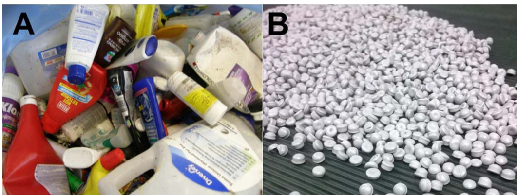
Figure 1. Collected and sorted HDPE packages (A) and granulated HDPE (B). [Color figure can be viewed in the online issue, which is available at wileyonlinelibrary.com .]
